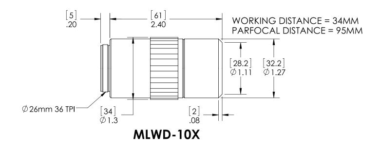
DIMENSIONS SHOWN ARE INCHES [MILLIMETERS] DIMENSIONS SHOWN FOR REFERENCE ONLY.
